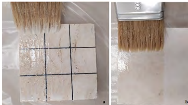
Fig. 3. Water-repellent chemical application process a) water-based water-repellent chemical application, b) solvent-based water-repellent chemical application
