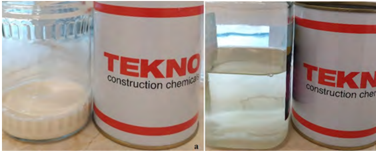
Fig. 2. Appearance of water-repellent chemicals a) water-based water repellent, b) solvent-based water repellent
