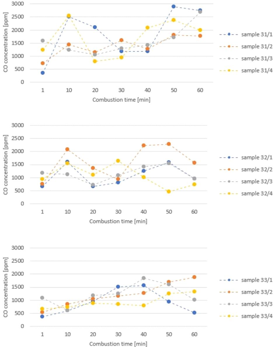
Fig. 2. CO emission during hard-coal combustion
