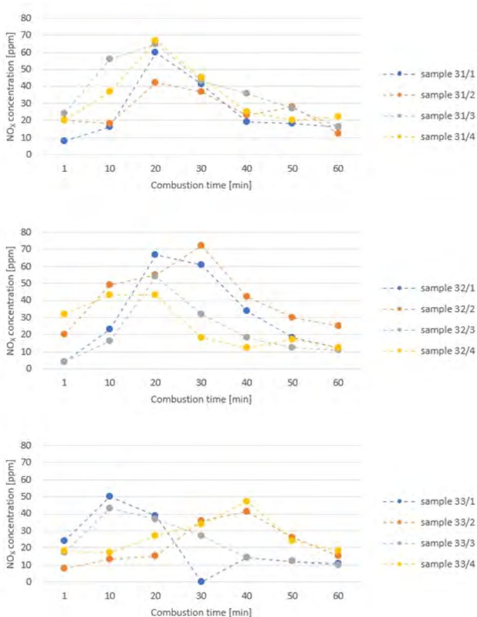
Fig. 4. NO<sub>x</sub> emission during hard-coal combustion
