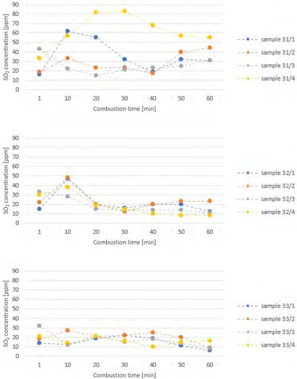
Fig. 5. SO<sub>2</sub> emission during hard-coal combustion
