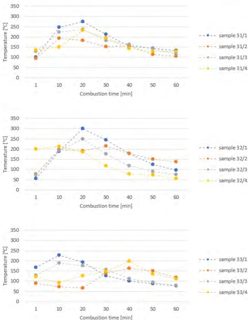
Fig. 6. Temperature of emitted gases during hard-coal combustion
