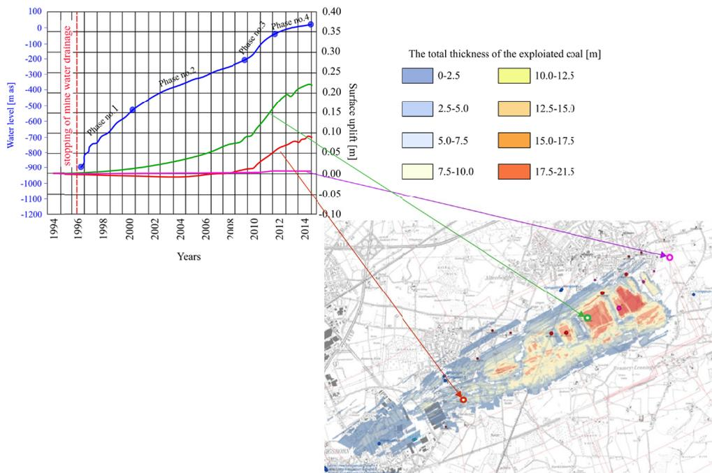
Fig. 1. Example land surface uplift during the flooding of the Königsborn mine (own study based on RAG materials)
