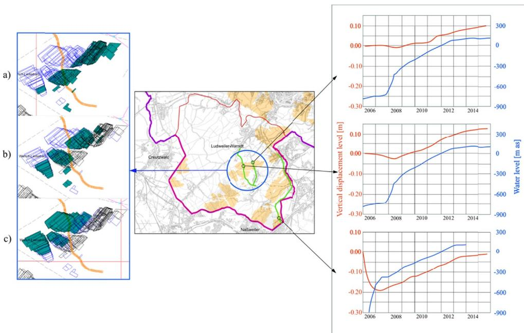
Fig. 2. Example land surface uplift during the flooding of the Warndt mining district (own study based on RAG materials)
