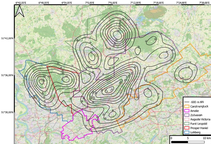
Fig. 5. The predicted distribution of uplift within the analysed area assumes a mining water level rise up to  $-600$  m a.s.l.
