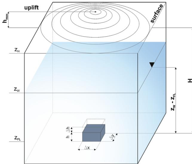
Fig. 3. Graphical explanation of the mathematical model of uplift caused by rising mining water levels [33]
