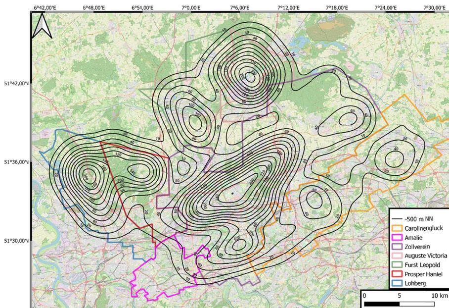
Fig. 6. The predicted distribution of uplift within the analysed area assuming mining water level rises up to  $-500$  m a.s.l.
