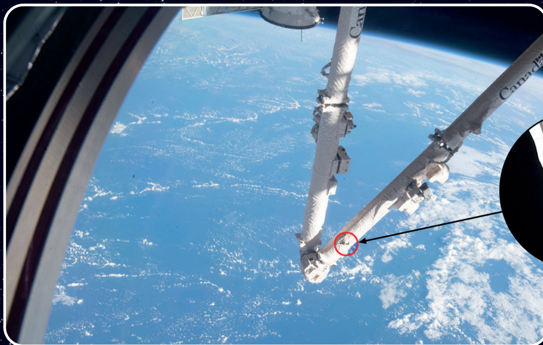
The Canadarm2 robotic arm punctured by space junk, NASA
