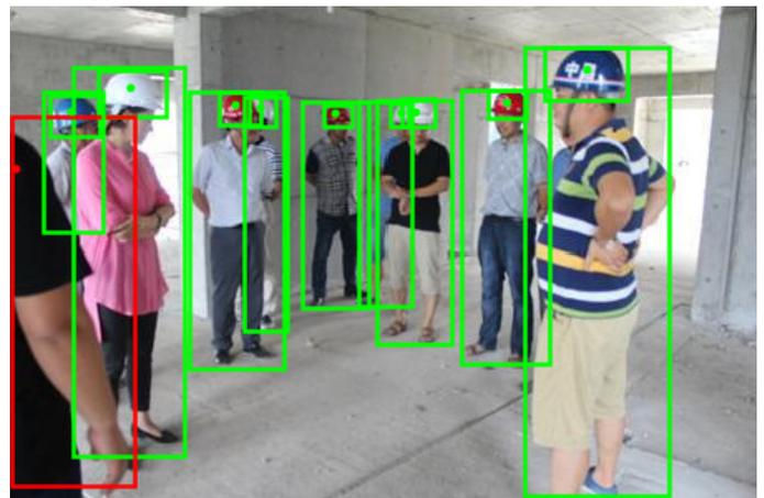
(f) failure in head center detection for partially visible person
