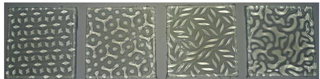
**Fig. 5.** Real samples laminated in the glass-EVA-modified ETFE material system. Surface modification patterns as in Fig. 4. From the left: flowers, dots and spots, leaves, camo.
