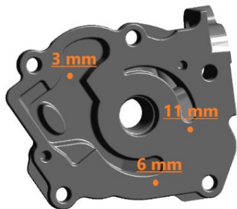
Fig. 2. Water pump cover geometry – view from MAGMASoft®
