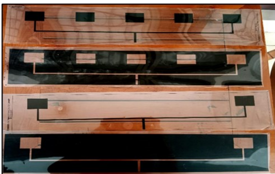
Fig. 11. Negative film in the photo etching process
