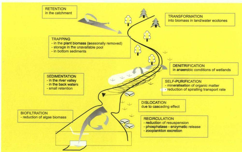
An example of synergistic interactions between different processes to enhance a river basin's capacity for self-purification
