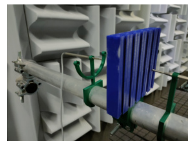
Fig. 4. Measurement stand scheme in the semi-anechoic acoustic chamber.
