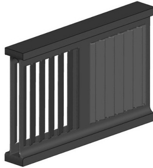
Figure 4: The geometrical model of the tested louvered fin.
