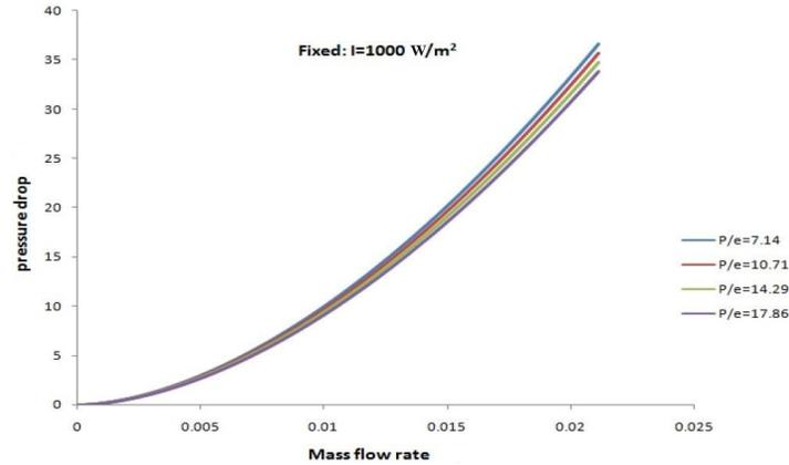
Figure 12: Variation of pressure drop ( $\Delta p$ ) with mass flow rate ( $\dot{m}$ ).
