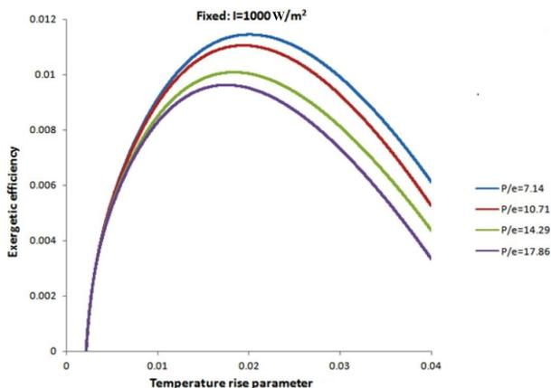
Figure 9: Variation of exergetic efficiency ( $\eta_{ex}$ ) with temperature rise parameter ( $\Delta T/I$ ).
