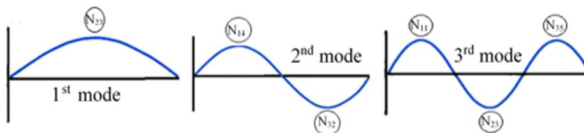
Fig. 1. The first three mode shapes
