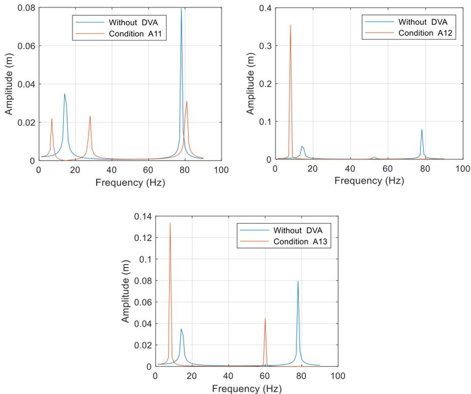
Fig. 4. Comparison of amplitudes between without and with DVA for conditions  $A_{11}$ ,  $A_{12}$  and  $A_{13}$
