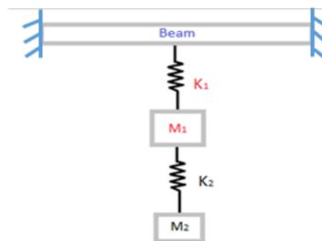
Fig. 3. Schematic representation of a beam structure attached with two DVA
