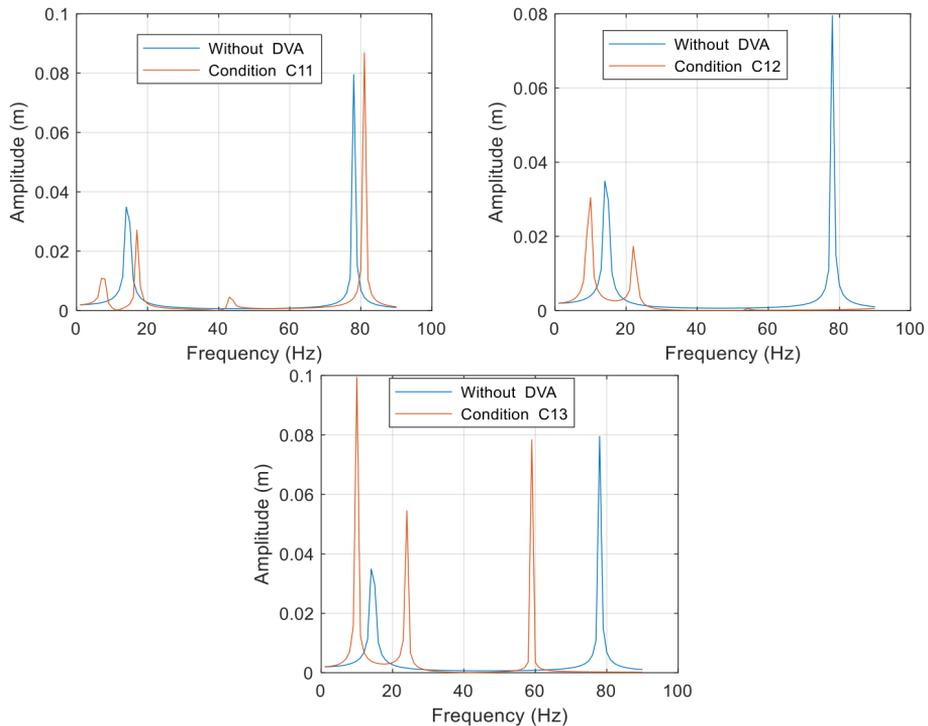
Fig. 7. Comparison of amplitudes between without and with DVA for conditions C<sub>11</sub>, C<sub>12</sub> and C<sub>13</sub>
