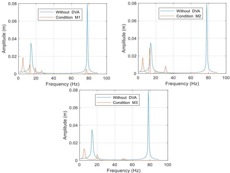
Fig. 13. Comparison of amplitudes between the cases without and with DVA for conditions  $M_1$ ,  $M_2$ , and  $M_3$
