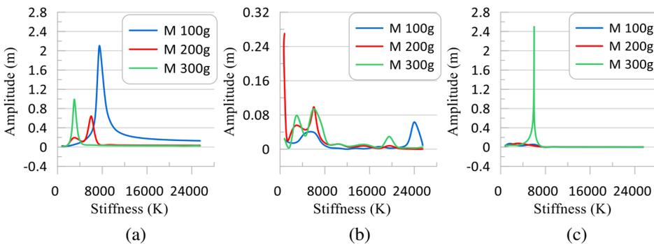
Fig. 15. The influence of stiffness on harmonic responsiveness for three mode shapes (a, b, and c)
