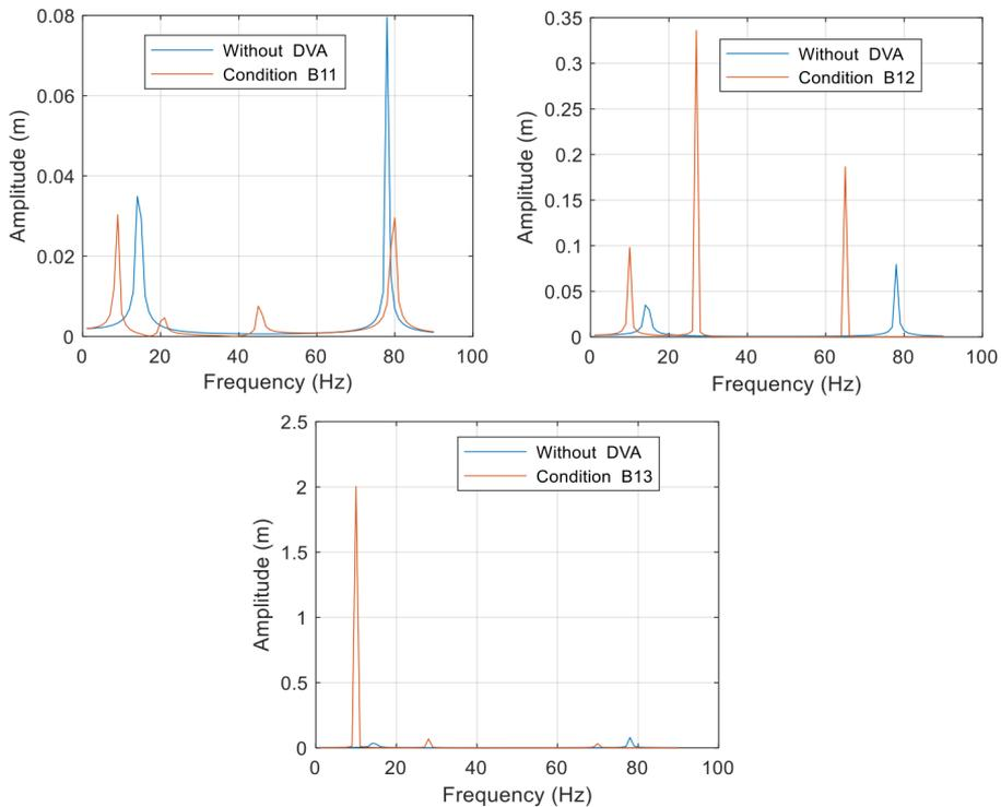
Fig. 5. Comparison of amplitudes between without and with DVA for conditions B<sub>11</sub>, B<sub>12</sub> and B<sub>13</sub>
