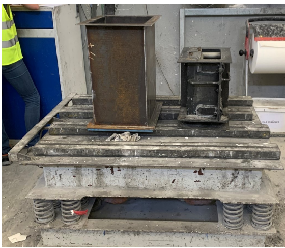
Fig. 1. Moulds on the vibrating table
