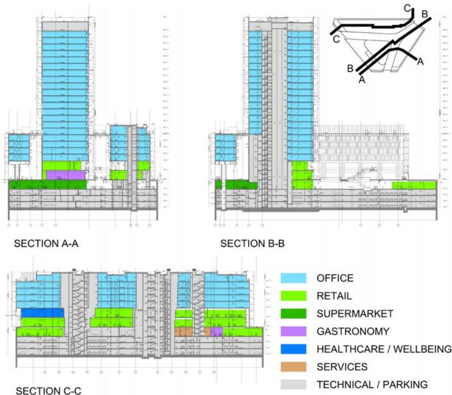
Fig. 8. Functional saturation of the complex; source: Kuryłowicz & Associates
