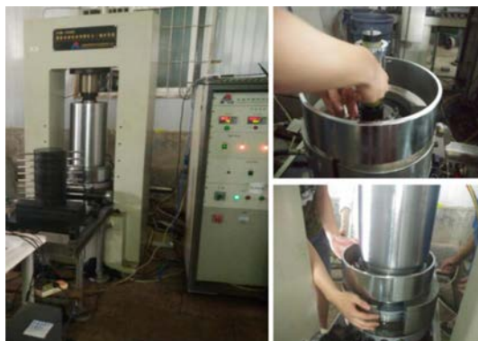
Fig. 8. TAW-3000 microcomputer servo-controlled triaxial rock testing machine
