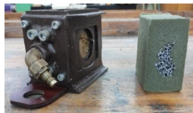
Fig. 2. The sampler used in testing the sand binding and the hardened shaped sample after its knocking out from the sampler
