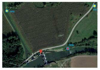
**Fig. 5.** Location of the fixed points currently employed for monitoring weir displacements; benchmark RP6 is situated on the damaged concrete sections of the weir; source: own elaboration based on Google Maps
