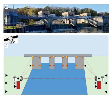
**Fig. 7.** Suggested approach for a control network of the weir: a) view of the structure, b) draft of the fundamental alterations in the geometry and setup of the control network; source: own elaboration, phot.: *L. Saloni*
