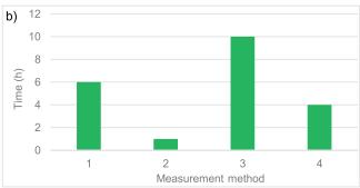
**Fig. 2.** Comparison of the applied methods in terms of: a) data acquisition time (h), b) point cloud development time (h), c) the number of people necessary to perform the measurement; measurements methods: 1 = photogrammetry UAV, 2 = airborne laser scanning (ALS), 3 = terrestrial laser scanners (TLS), 4 = angular-linear measurement; source: Pasternak (2023), modified
