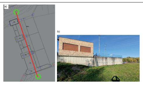
**Fig. 4.** Baseline for the weir: a) design of the installation, b) area where construction work was left unfinished (no possibility of stabilising an observation post of the suitable height); source: own elaboration, phot.: *L. Saloni*
