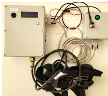
Fig. 3. Proprietary breath recording system using a piezoresistive sensor.
