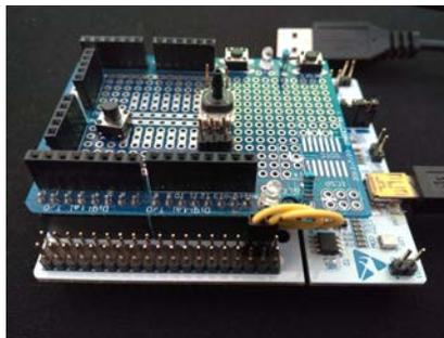
Fig. 2. Proprietary pressure measurement system using the MEMS system based on STM32 Microcontroller.
