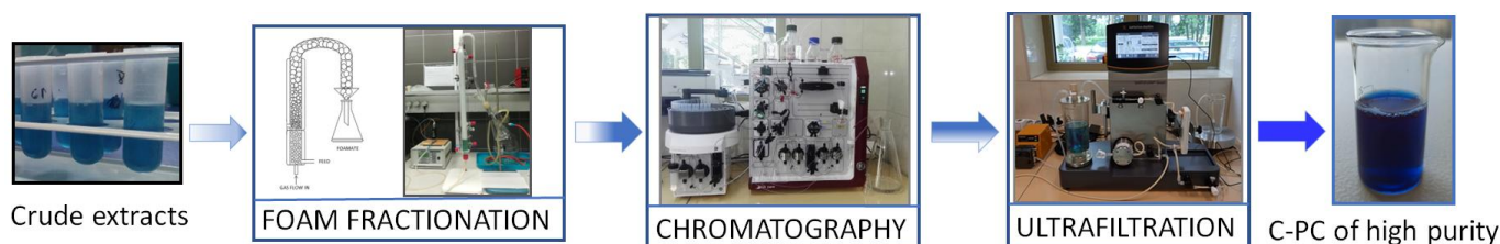
Figure 6. A three-stage method to achieve a C-PC of a high degree of purity.
