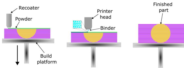
Fig. 1. Scheme of the process of 3D printing of molding sands using the binder jetting method [3]
