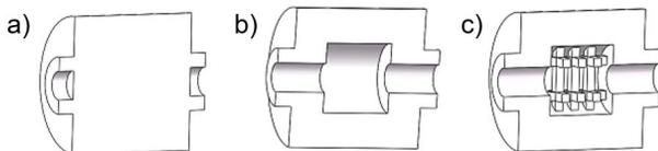
Fig. 5. Diagram of cores: a) solid b) with a cavity c) with a truss structure [33]
