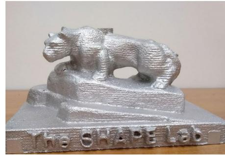
Fig. 3. Casting with a visible stepping effect on the surface [20]
