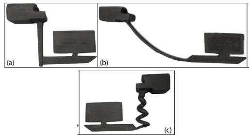
Fig. 6. Types of tested sprues a) classic b) parabolic c) spiral [38]
