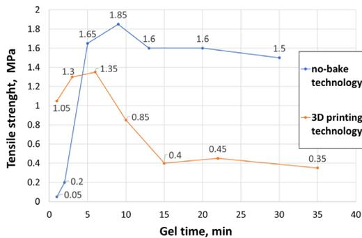
Fig. 2. The influence of gel time on tensile strength tested after 24h of hardening [20]
