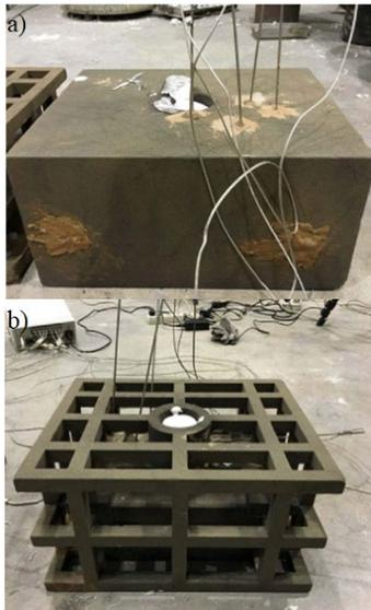
Fig. 4. Printed molds: a) classic type of mold b) mold with cavities (shell-truss mold) [4]
