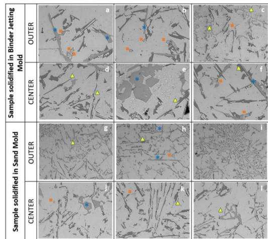
Fig. 7. Microstructures of the samples, outer layers of the casting (a-c) in the mold created in the binder jetting technology, and the center of the casting (d-f), the outer layer obtained in the sand mold (g-i) and the middle part of the casting (j-l), \* - phase Si, ■ -  $\text{AlCu}_2$ , ▲ -  $\text{Al-Fe-Si}$  [46]
