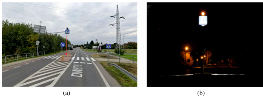
Fig. 3. Daytime view of pedestrian crossing no. 3 with dedicated pedestrian crossing lighting on a single-lane two-way street with a separator lane without additional street lighting (a) and visibility of a pedestrian in dark-colored clothing waiting to cross the street (b)
