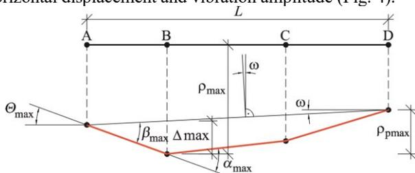
**Fig.4.** Symbols for the displacement of foundations acc. to EC-7 [39]
