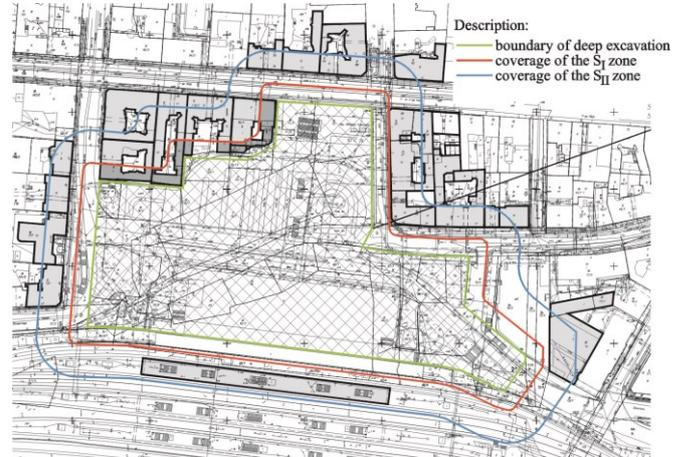
Fig.14. Impact zones of the excavation
