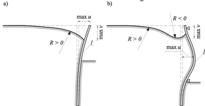
**Fig. 1.** Shape of soil settlement profile within deep excavation:
