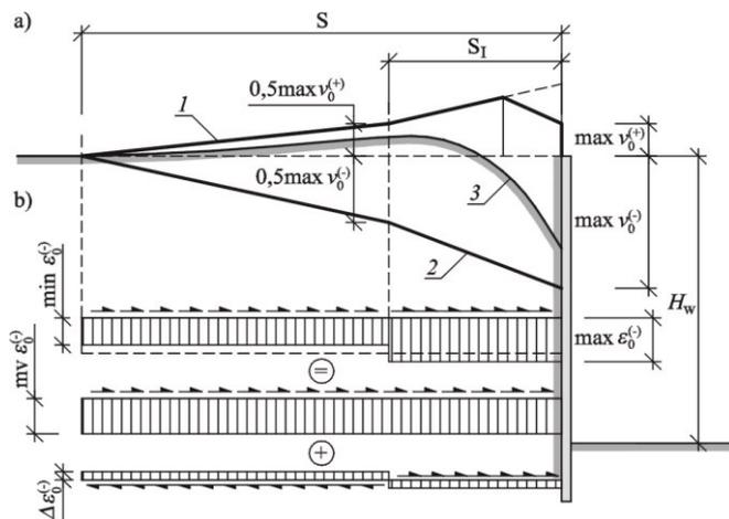
Fig.11. Simplified distributions of vertical displacements and deformations of the ground near the deep excavation [30]: a) vertical displacements, b) ground deformations; 1 – extreme distribution of negative displacements, 2 – extreme distribution of positive displacements, 3 – average distribution of displacements
