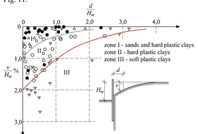
Fig.9. Measurement results for ground settlement acc. to Peck [52]
