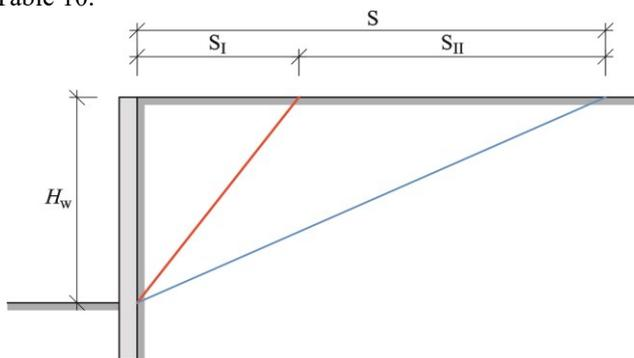
Fig.13. The area of impact zones of the excavations  $S_I$  and  $S$  [30]
