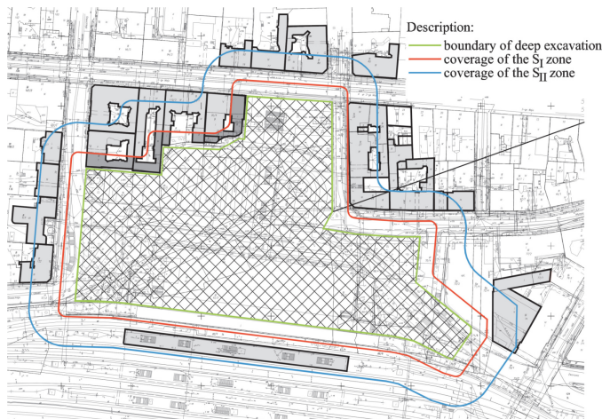
Fig. 14. Impact zones of the excavation
