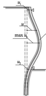
**Fig.12.** Horizontal displacement of the support wall: 1 – excavation support system after deformation,  $u_1$ ,  $u_2$  – wall displacements caused by installation of supports in stages
