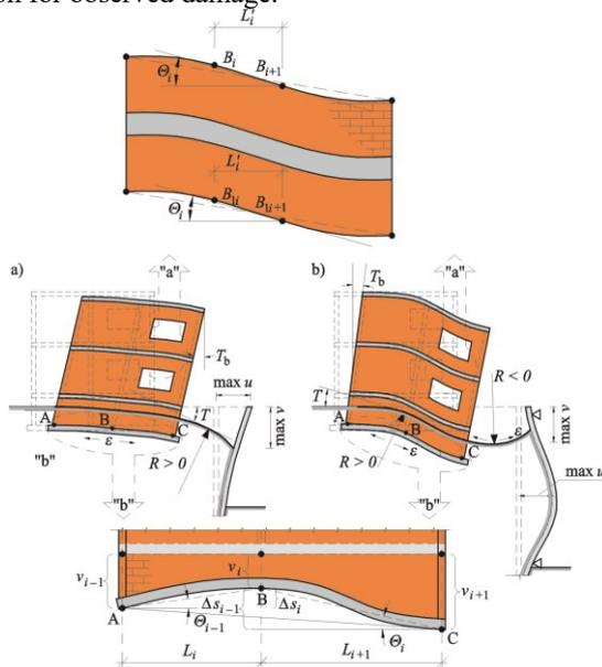
**Fig.3.** Parameters typical for soil deformation near deep excavation for various schemes: a) the non-supported cantilever scheme, b) the supported scheme, "a" – shear strains of lintel or spandrel area, b) deformation at the level of foundation
