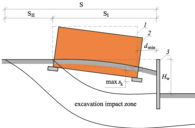
**Fig. 7.** Maximum displacement of the structure acc. to [30]: 1 – state before commencement of construction works, 2 – state during construction works, 3 – support system of the excavation, S – impact area of the excavation,  $S_I$  – area of direct impact of the excavation,  $S_{II}$  – area of the secondary impact
