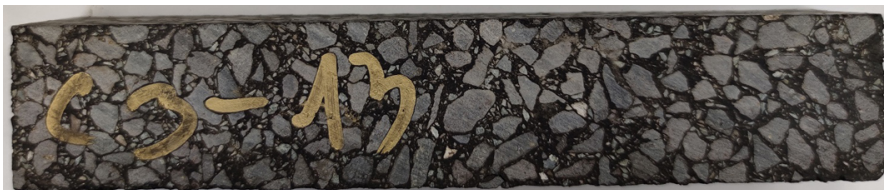
Fig. 3. Cross-section through a specimen of SMA-MA PMB 65/105-80 mixture
