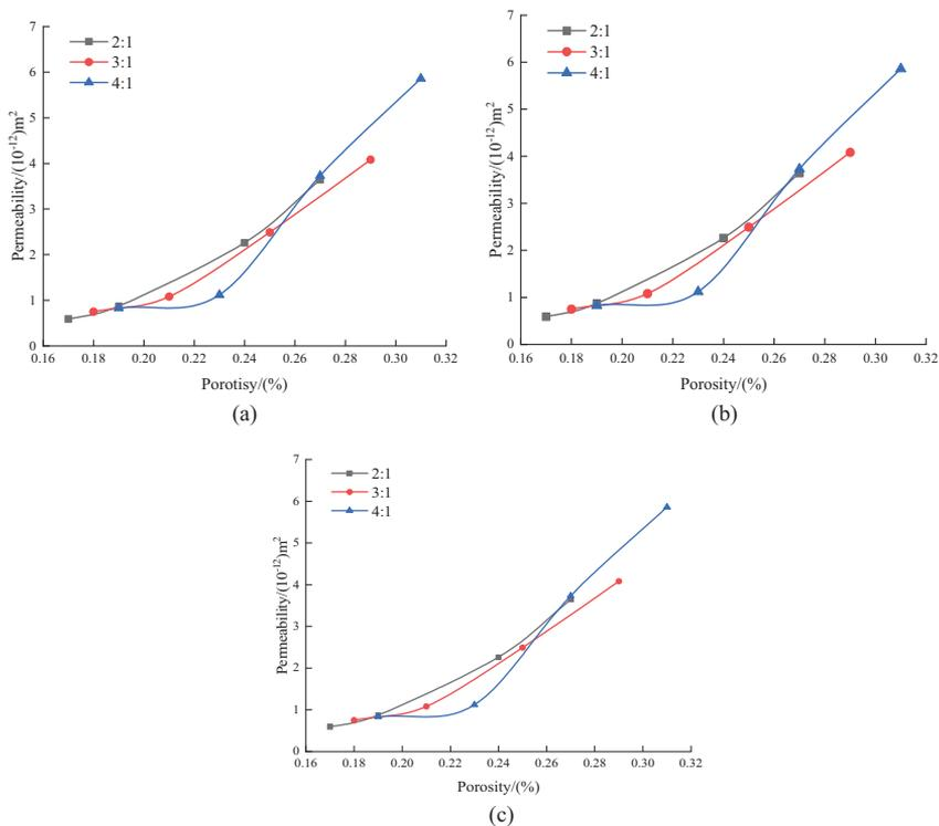
Fig. 6. Porosity-permeability relationship curve, wall rack: a) 3 MPa, b) 3.5 MPa, c) 4 MPa
