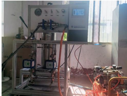
Fig. 5. Broken rock mass penetration test system
