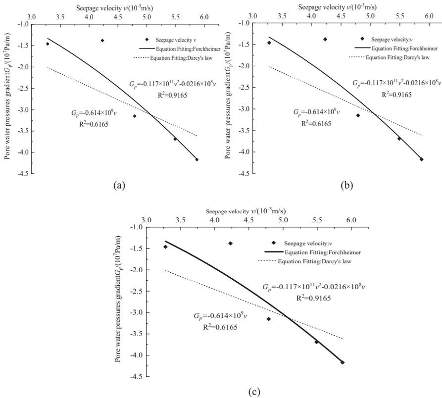
Fig. 8. The relation curve between pore pressure gradient and seepage velocity, scale of coarse and fine particles: a) 2:1, b) 3:1, c) 4:1
