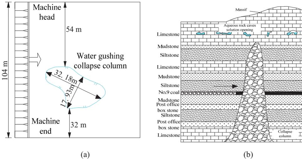
Fig. 1. Schematic diagram of the level profile of the fall column: a) Ichnography, b) Section plan
