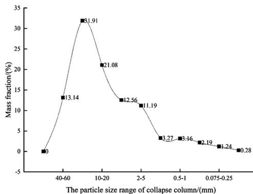
Fig. 2. Grain size distribution of the fall column
