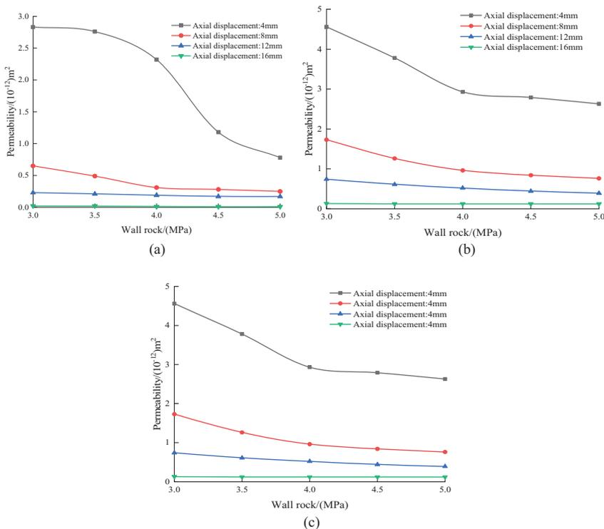
Fig. 7. Wai-pressure-permeability relationship curve, scale of coarse and fine particles: a) 2:1, b) 3:1, c) 4:1
