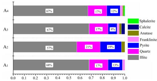
Fig. 4. Composition and proportion of fall column filling sample
