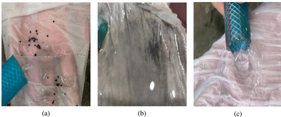
Fig. 9. Water evolution stage of broken rock mass: a) Initial percolation phase, b) Permeability phase, c) Pipe surge stage
