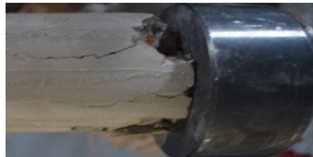
(b) Tensile failure
