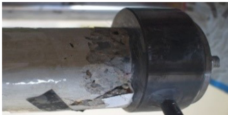
(a) Spalling failure
