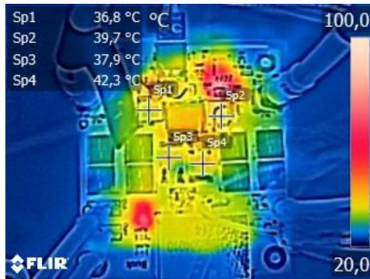
**Fig.7.** Results of the thermal imaging measurements of the converter at  $P_{out} = 400$  W,  $f_s = 400$  kHz and forced air flow with an ambient temperature of 20 degrees Celsius (measurement points Sp1, Sp2 indicates transistors and Sp3, Sp4 diodes).
