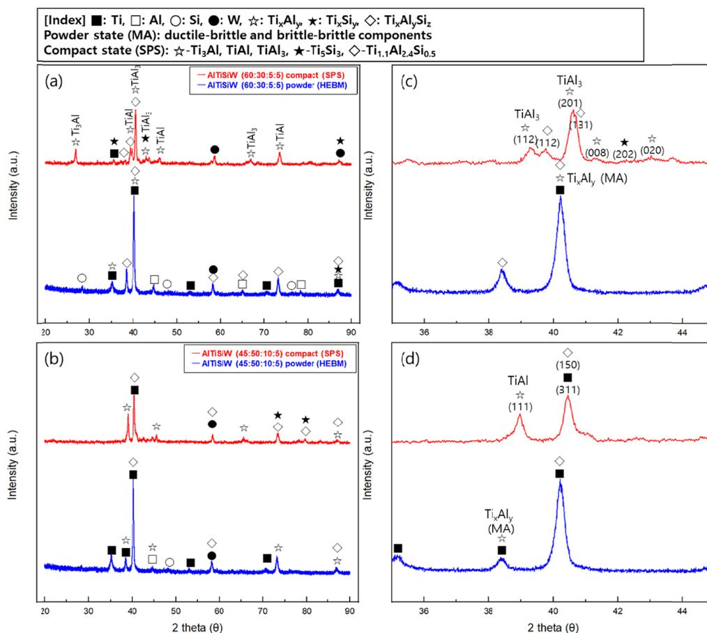
Fig. 1. XRD patterns of Al-Ti-Si-W alloys fabricated by high energy ball milling and spark plasma sintering: (a)  $Al_{60}Ti_{30}Si_5W_5$ , (b)  $Al_{45}Ti_{50}Si_{10}W_5$ , (c) and (d) magnification of peaks for major phases
