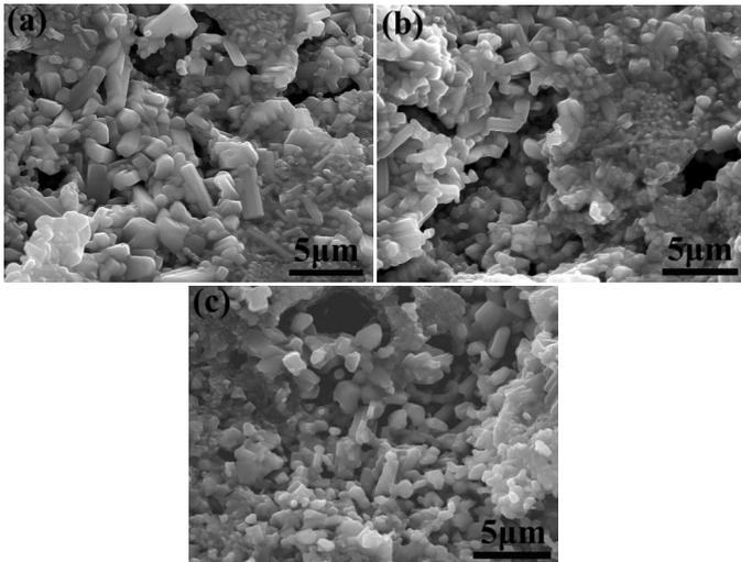
Fig. 8. SEM observations on the surfaces of Nb-Si-Ti-Cr-Al-Ta-Hf alloys with different Ho addition oxidized at 1373 K for 60 hours: (a) 0 Ho, (b) 0.1 Ho, (c) 0.2 Ho
