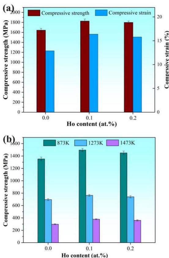
Fig. 4. Compressive properties of the Nb-Si-Ti-Cr-Al-Ta-Hf alloys with different Ho addition: (a) Compressive strength and strain at room temperature, (b) Compressive strength at elevated temperature
