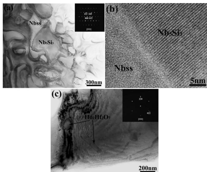
Fig. 3. TEM observations on the Nb-Si-Ti-Cr-Al-Ta-Hf alloy with 0.2 Ho addition: (a) Fine Nb/ $Nb_5Si_3$  eutectic structure, (b) Morphology of  $Ho_2Hf_2O_7$  particles (Inset images showing the SAED pattern of corresponding phases)
