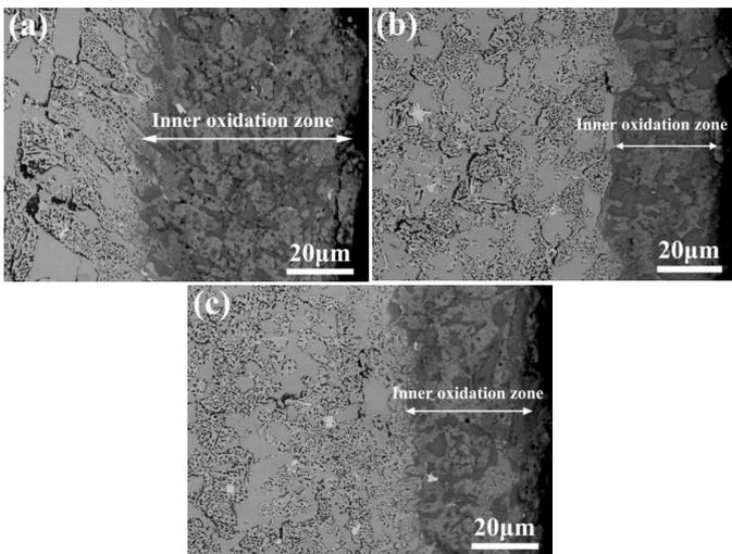
Fig. 9. SEM observations on cross-section of Nb-Si-Ti-Cr-Al-Ta-Hf alloys with different Ho addition oxidized at 1373 K for 60 hours: (a) 0 Ho, (b) 0.1 Ho, (c) 0.2 Ho
