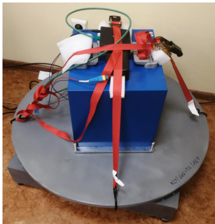
Fig. 17. The FOS6-02 on rotating platform prepared for the tests.
