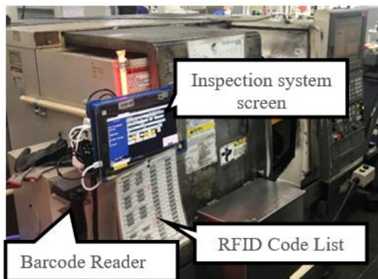
Fig. 18. Actual Industry 4.0's system in the CNC process
