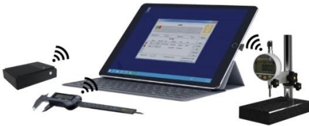
Fig. 16. Measuring system according to the IoT protocol
