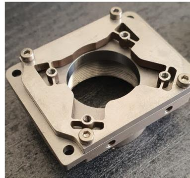
**Fig. 14.** The modified c-mount block with flexures.
