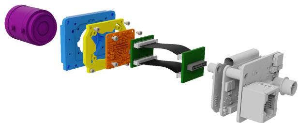
**Fig. 15.** The exploded view of the redesigned camera.
