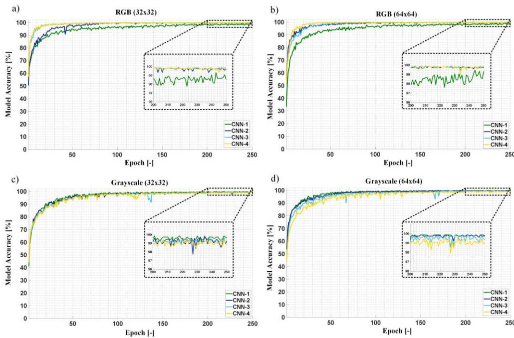
**Fig.10.** CNN models accuracy during the training process for different structures and input images: a) RGB (32x32), b) RGB (64x64), c) grayscale (32x32), d) grayscale (64x64) ( $\eta=0.0001, B=8, \gamma=0.5$ ).
