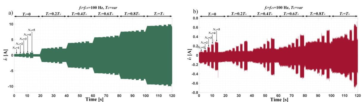
**Fig.4.** The waveforms of the (a)  $i_1$  and (b)  $i_2$  for  $T_L = \text{var}$ , rated supply voltage frequency ( $f_s=f_{sN}=100$  Hz), and momentary short-circuiting of 1 to 5 turns in the PMSM stator winding.
