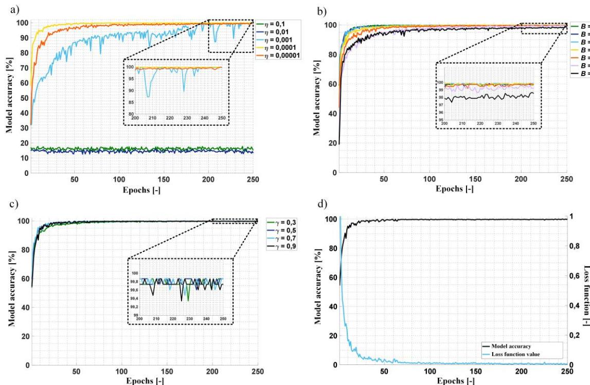
**Fig.14.** CNN models accuracy during the training process for different input images and network structures: a) CNN-1, b) CNN-2, c) CNN-3, c) CNN-4 ( $\eta=0.0001, B=8, \gamma=0.5$ ).
