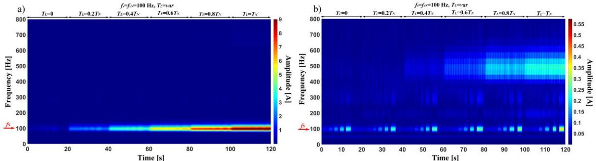
**Fig.5.** CWT scalograms of the (a)  $i_1$  and (b)  $i_2$  for  $T_L = \text{var}$ , rated supply voltage frequency ( $f_s=f_{sN}=100$  Hz), and momentary short-circuiting of 1 to 5 turns in the PMSM stator winding.
