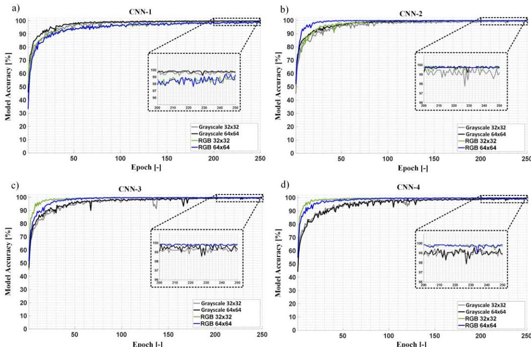
**Fig.11.** CNN models accuracy during the training process for different input images and network structures: a) CNN-1, b) CNN-2, c) CNN-3, d) CNN-4 ( $\eta=0.0001, B=8, \gamma=0.5$ ).
