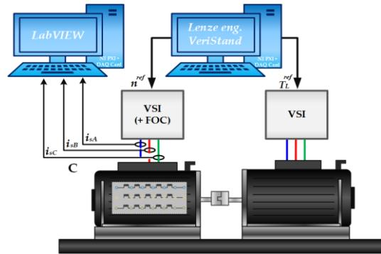
**Fig.3.** Simplified block diagram of the test bench.
