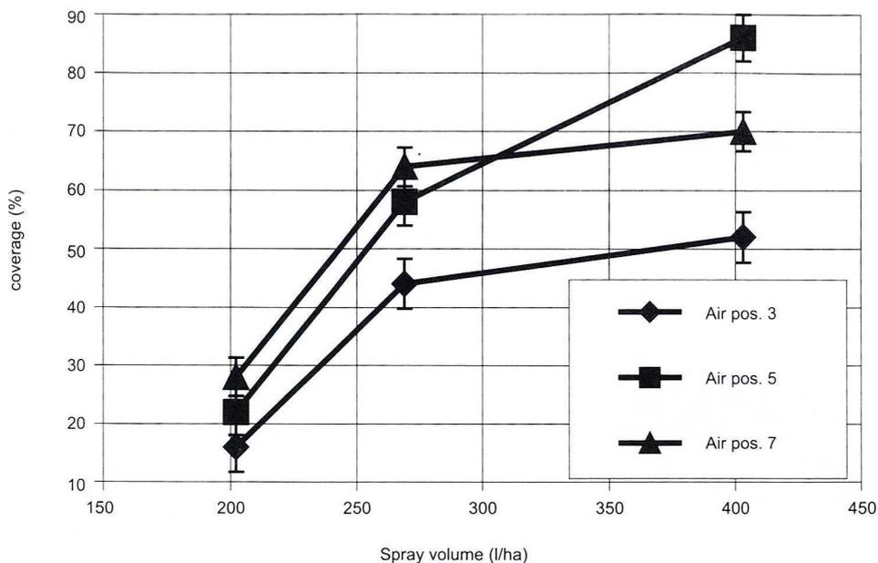
Fig. 2. Spray coverage of plant half the height (level II) for different air settings and spray volumes Q
