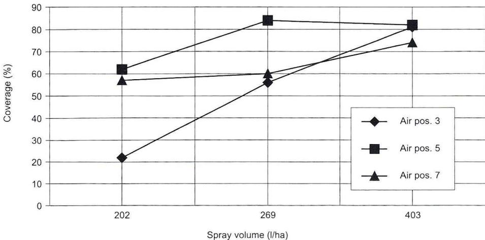
Fig. 1. Spray coverage of winter wheat tops (level I) for different air settings
