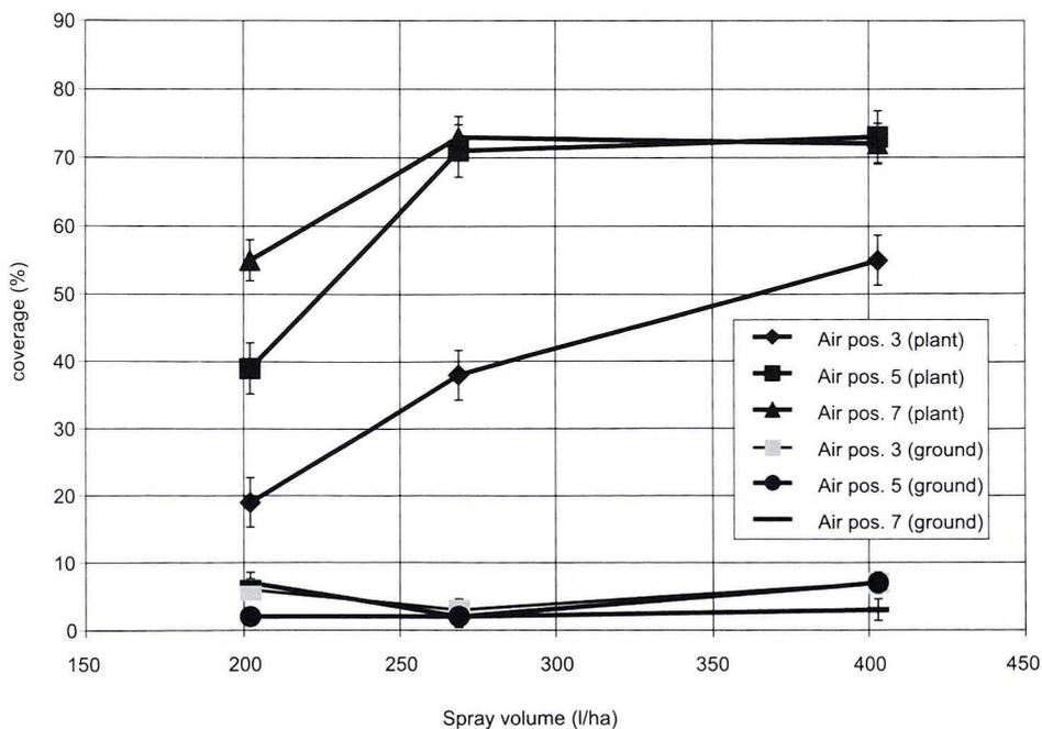
Fig. 3. Mean spray coverage of whole plant and spray coverage of the ground for different air settings and spray volumes Q
