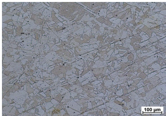
Fig. 1. Microstructure of annealed brass, magnification 100x
