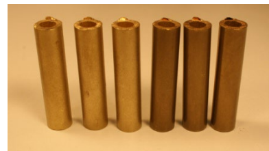
Fig. 3. Samples after the annealing process, visible burrs
