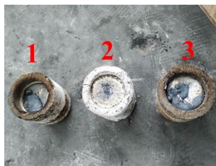
Fig. 15. Risers cut from the casting
