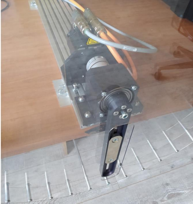
Fig.3. The servo system
