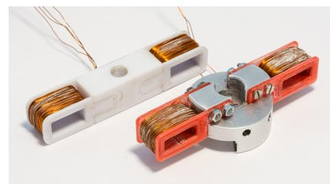
Fig. 4. 3D printed prototypes of in-house built torsional excitation coils
