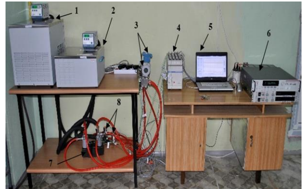
Fig. 1. The picture of the experimental setup: 1 – calibration bath of the cold side, 2 – calibration bath of the hot side, 3 – hot and cold side pressure transducers, 4 – ice point reference, 5 – LabVIEW control program, 6 – Keithley digital multimeter, 7 – investigated minichannel heat exchanger with insulation, 9 – hot and cold side flow meters.
