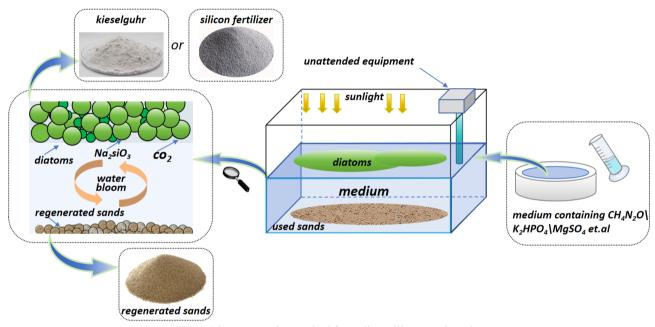
Fig. 1. Bio-regeneration method for sodium silicate used sands
