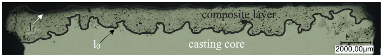
Fig. 4. Microstructure of carbon cast steel after heat treatment (S2)
