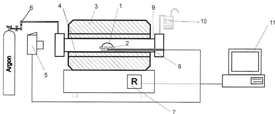
Fig. 1. Schematic view of the measuring apparatus: 1 – drop of liquid metal; 2 – substrate; 3 – high-temperature furnace; 4 – heating elements; 5 – CCD camera; 6 – gas delivery system; 7 – furnace work regulator; 8 – loading system with thermoelement; 9 – reactor; 10 – gas outlet system; 11 – PC computer.
