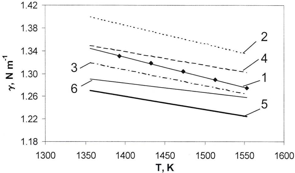
Fig. 7. A comparison between the liquid copper surface tension measurements and the literature data in the temperature range 1356-1553 K (1 - present work, 2 - [2], 3 - [20, 22], 4 - [21], 5 - [23], 6 - [24]).
