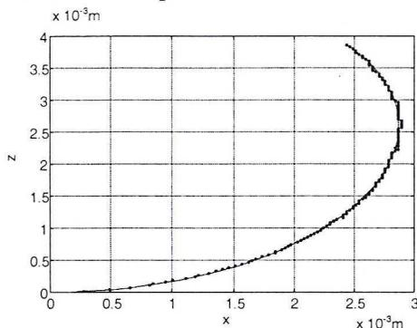
Fig. 6. A copper drop shape at 1433 K (the full line represents the solution of the system of differential equations (12-14) for  $b^*=0.30993 \cdot 10^{-2}$  m and  $B^*=0.59414 \cdot 10^5$  m<sup>-2</sup>)
