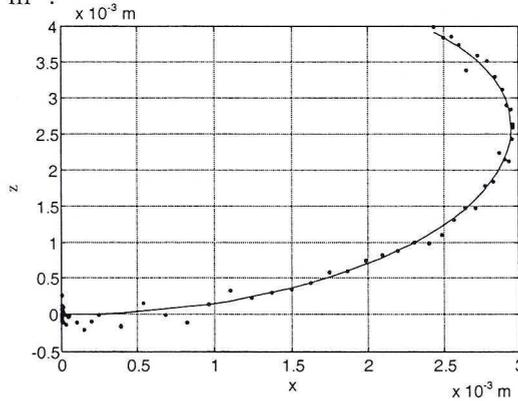
Fig. 5. A drop profile ( $b^*=0.32826 \cdot 10^{-2}$  m,  $B^*=0.78357 \cdot 10^5$  m<sup>-2</sup>) obtained by the estimation of the parameters describing the drop shape and size on the basis of the test points
