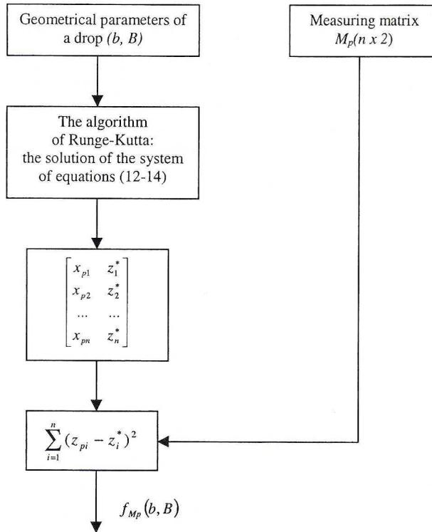
Fig. 4. The algorithm of the function  $f_{Mp}(b, B)$  value calculating appearing in the optimisation problem (10)
