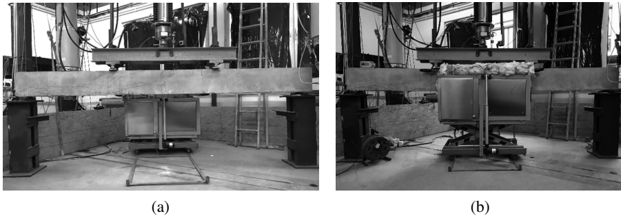
Fig. 3. Test setup (a) subjected to loading (b) subjected to both loading and heating
