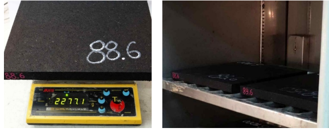
Fig. 3. UBM samples no. 88.6 during the ageing test with high temperatures: a) sample during the mass measurement; b) samples in the climatic chamber
