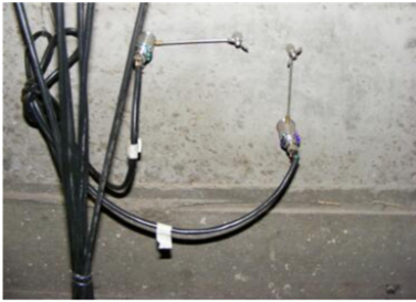
Fig. 23. Strain monitoring measurement points
