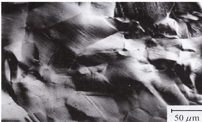
Fig. 4. Optical micrograph of the specimen surface after strain of 0.045. At this strain de_s/dw_p has the maximum
