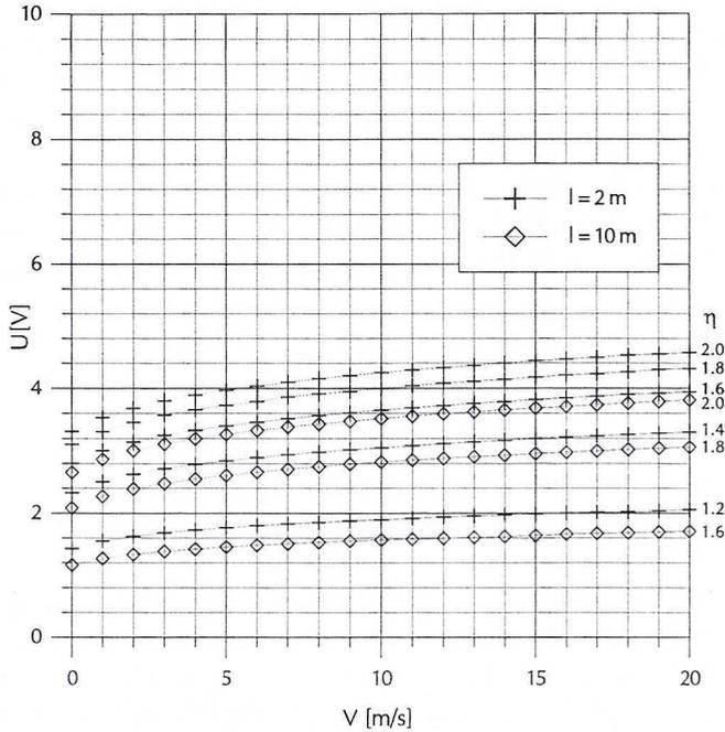
Fig. 7. Static characteristics for the two-point circuit
