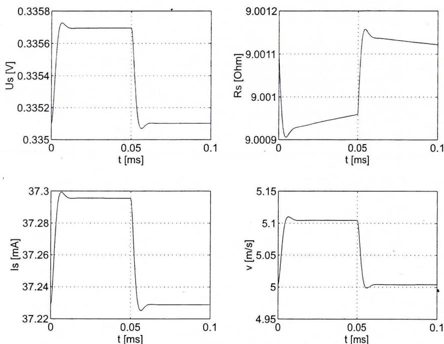
Fig. 4. Simulation results for the step function of flow velocity
