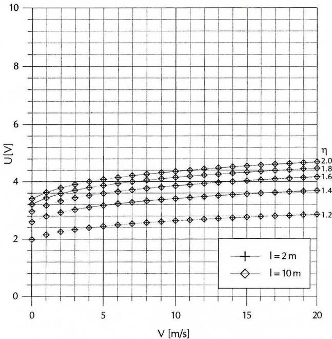
Fig. 6. Static characteristics for the four-point circuit
