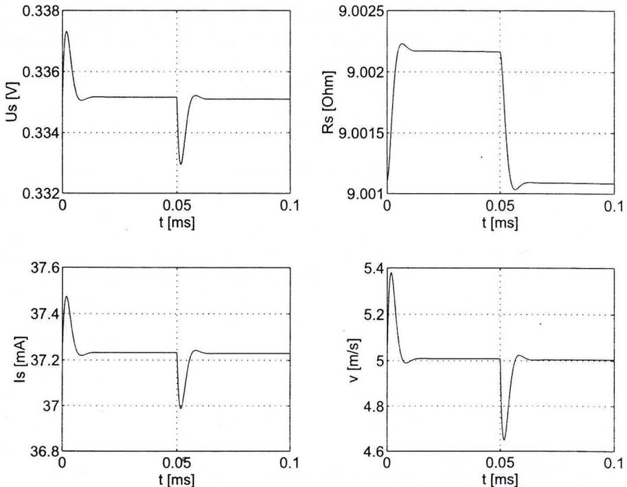
Fig. 3. Simulation results for the step function of the offset voltage
