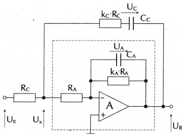
Fig. 2. Equivalent circuit of the PI controller
