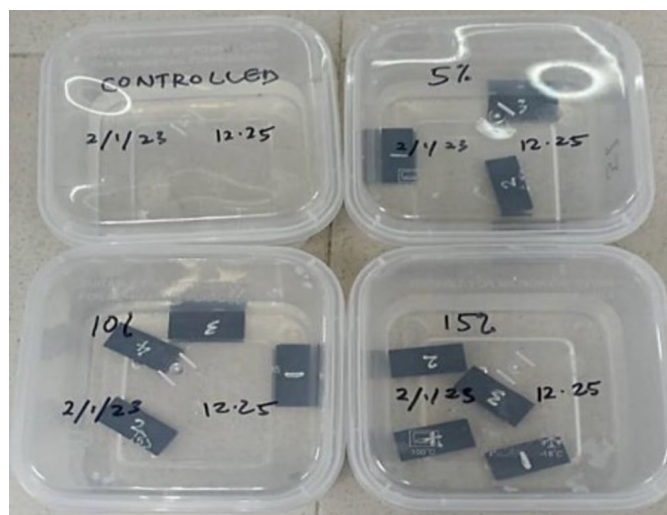
Fig. 3. Submerged PLA/Carbon CCH Composite Samples for Water Absorption Test
