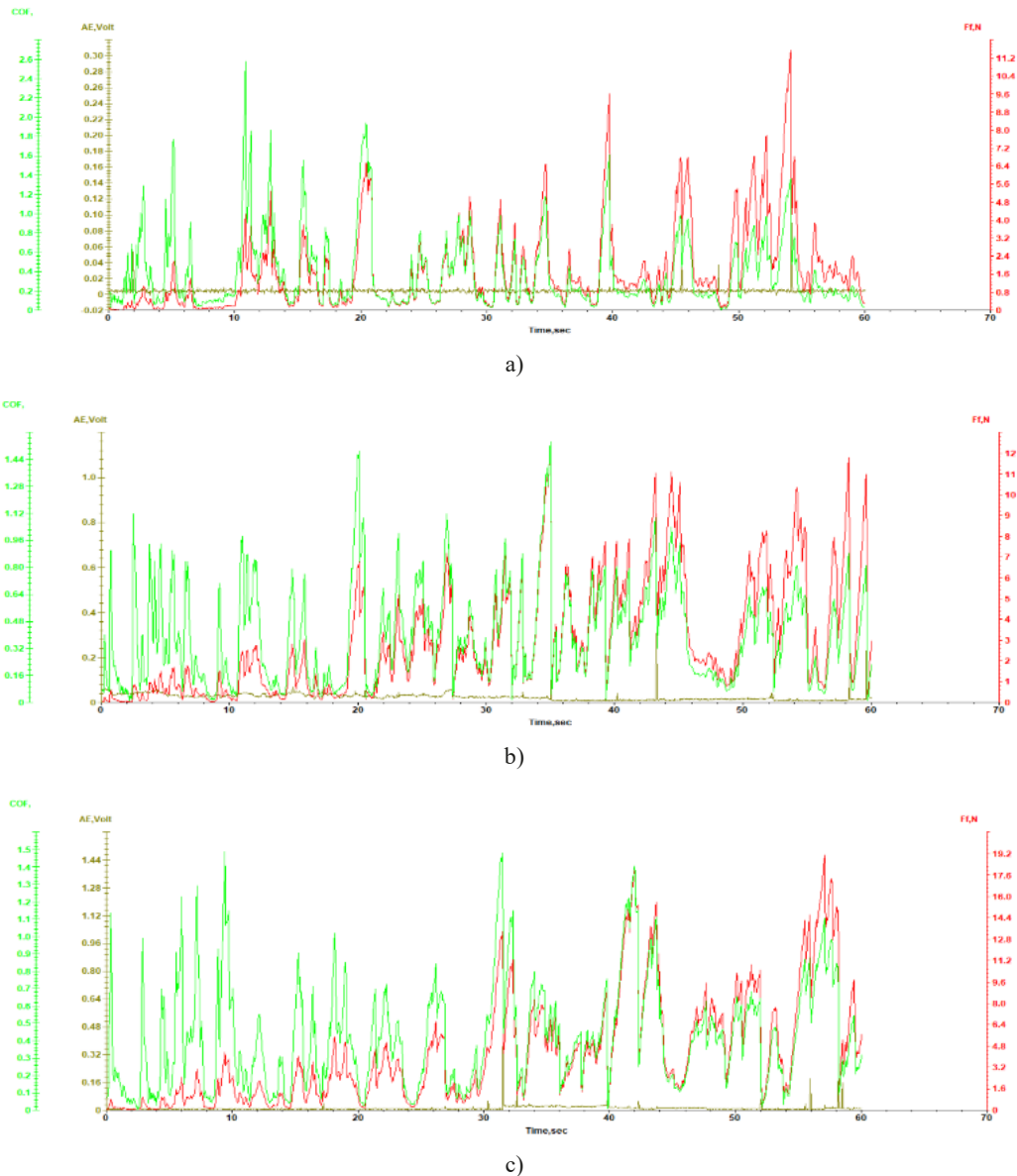
Fig. 5. The time variation diagrams of friction coefficient (COF, green) – friction force (Ff, red) – acoustic emission (AE, brown) for WC-TiC coatings, resulted after the scratch tests with a progressive load of: a) 10 N; b) 15 N; c) 20 N
