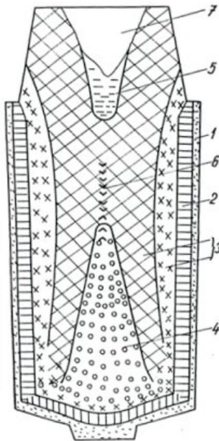
Fig. 1. Scheme of the structure in the ingot Area 1 Thin outer layer of fine, very clear polyhedral grains; Area 2 Columnar long axis, still very clear crystals; Area 3 Thick polyhedral grains; Area 4 Globular grains transformed into pyramid shape in bottom part of ingot; Area 5 Small zone just under the head of ingot; Area 6 Minimal homogeneity; Area 7 Head of ingot with shrinkage [23]
