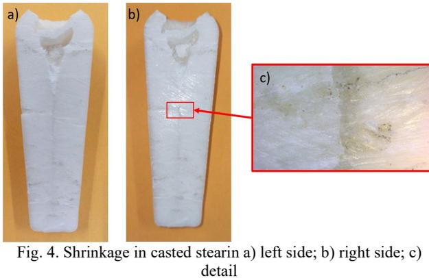
Fig. 4. Shrinkage in casted stearin a) left side; b) right side; c) detail
