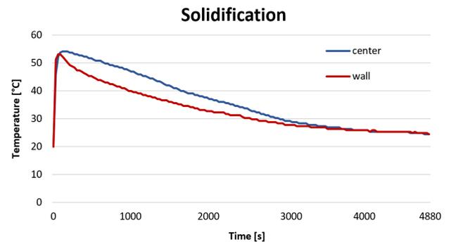
Fig. 3. Dependence of temperature on time during the cooling of the ingot
