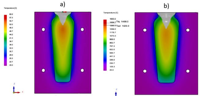
Fig. 5. Solidification process a) Stearin; b) high carbon steel.
